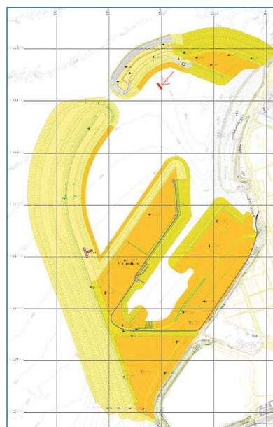
Figure 4 Top view of the Maasvlakte 2 project under construction. The coloured areas are being reclaimed with different sand types. Red arrow indicates location of TSHD (trailer suction hopper dredger) Oranje (see Figure 5) (courtesy PUMA)
