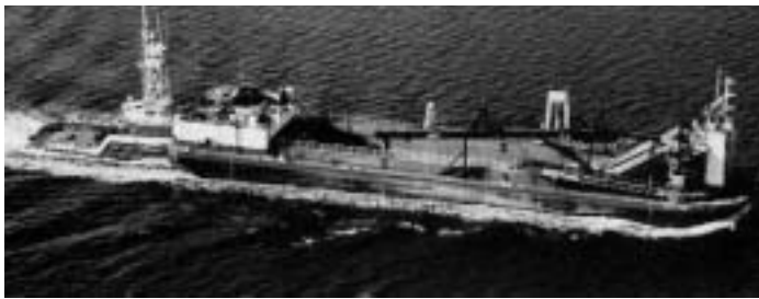
3,900 cubic-meter capacity hopper dredge Sandy Hook
